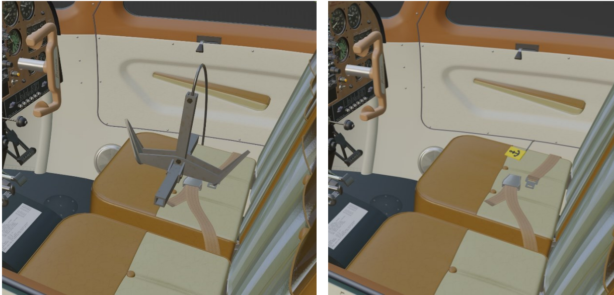
Figure I-6: Anchor Left: Available. Right: Deployed
